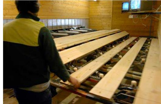
Visual and mechanical stress grading is carried out to provide C16 timber
